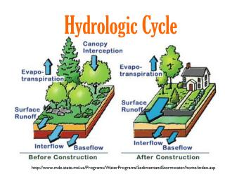
The hydrology of a site changes during the clearing and grading that occurs during construction.
