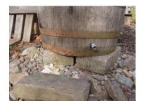
Prepare a level area to place the barrel. Some stone or cinder blocks work well
